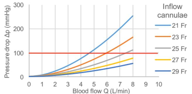
**Fig. 2.** The simulation result on created model of the pressure drop according to the EBF for inflow cannulas
