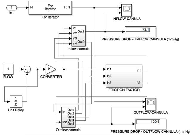
Fig. 1. System diagram of the cannula model in the ECMO system.
