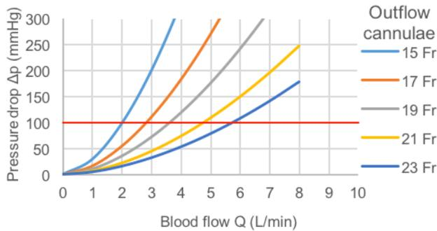
**Fig. 3.** The simulation result on created model of the pressure drop according to the EBF for outflow cannulas
