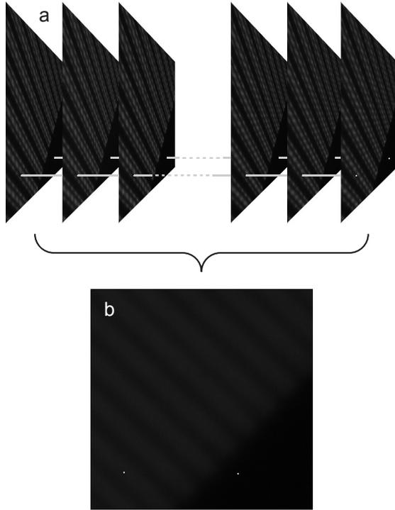
Fig. 2 Illustration of the mean of the whole image stack into the one image. (a) represents the stack of the raw SIM images acquired by the system described in chapter 3. Gray lines correspond to the two hot pixels which appear in all images in the stack. Image (b) is the mean image calculated from the full stack (a) containing two significant hot pixels.
