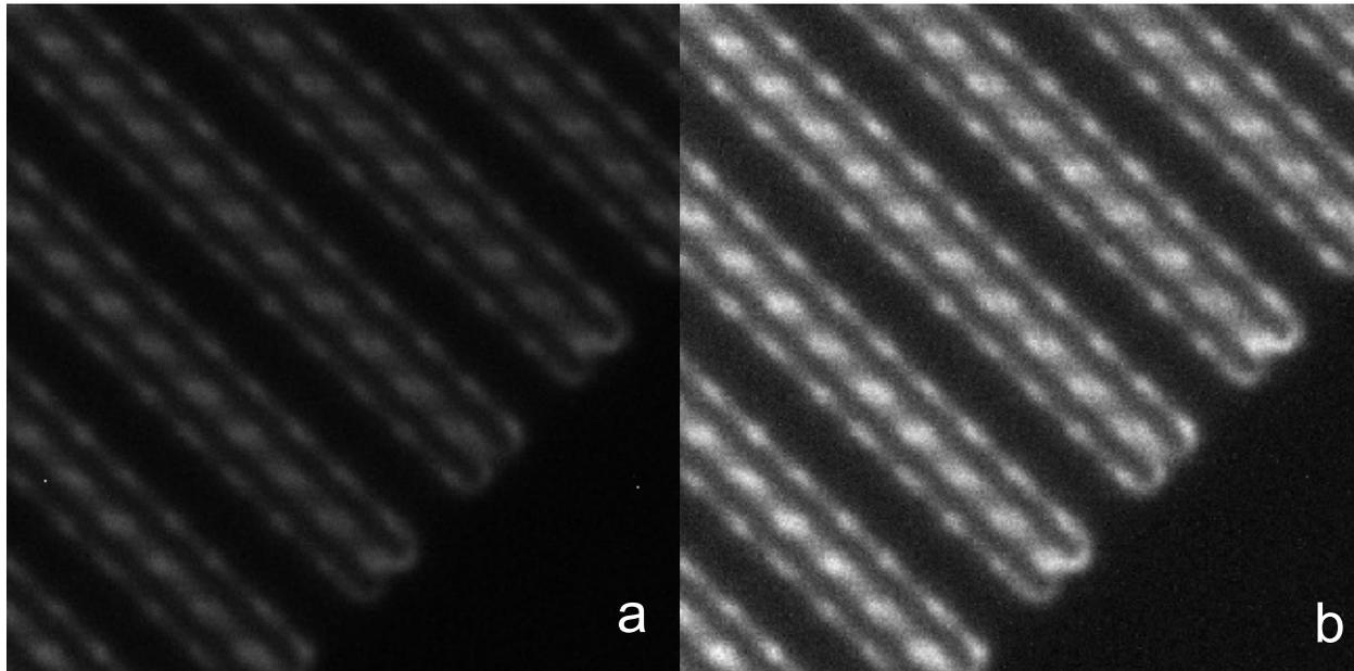
Fig. 5 The result of hot pixel detection and suppression. Both images represent the ROI of sum of whole stack normalized according the highest value in the image. Image (a) contains two significant hot pixels, which dramatically decrease the dynamic range. Image (b) shows the result of our algorithm.
