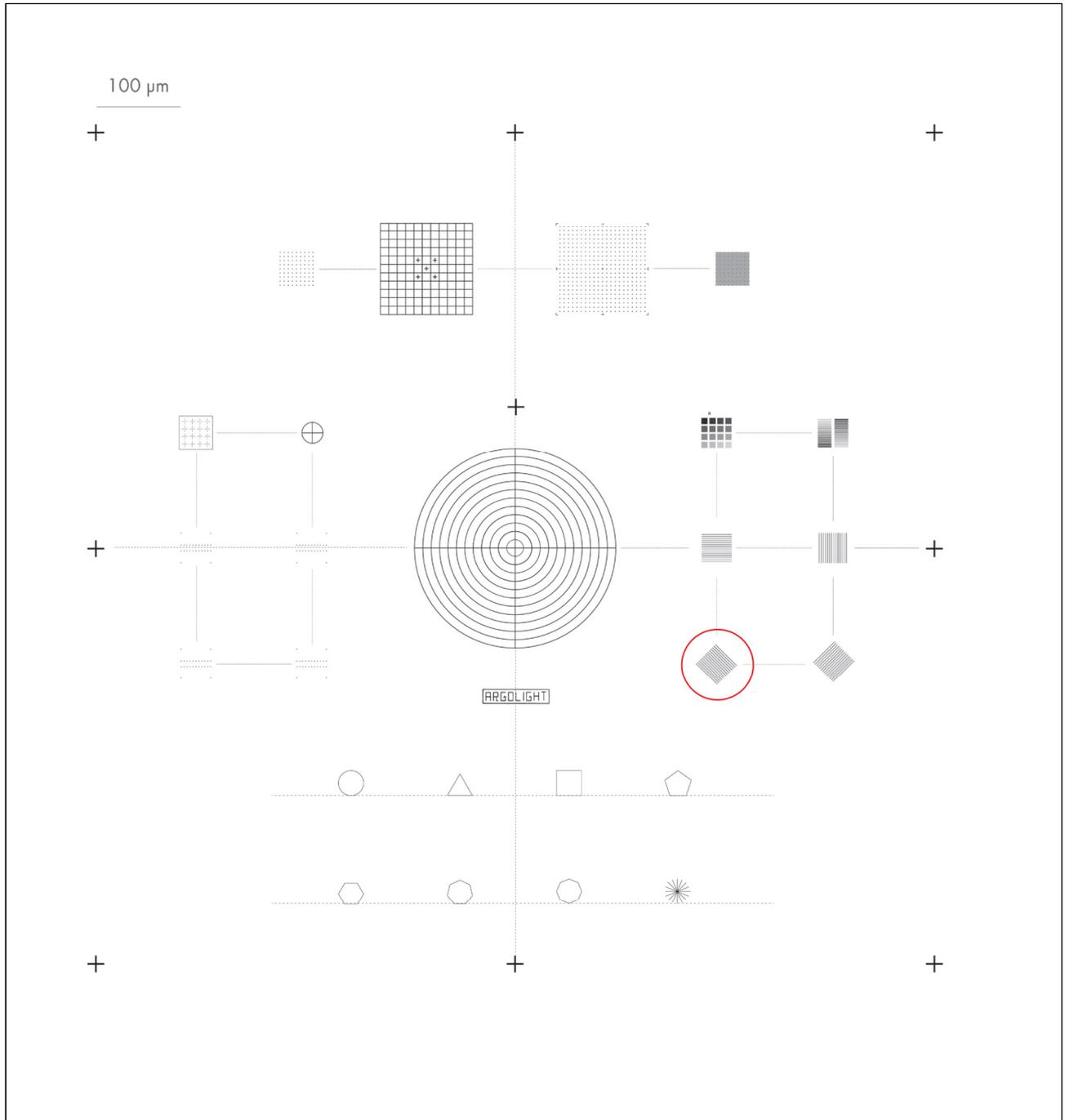
Fig. 6 Patterns overview. Matrix of rings, grid, 2D matrix of rings, matrix of rings on a background, matrix of crosses, meridians of a sphere, repositioning crosses, 4x4 intensity, 2x16 intensity, 3D crossing stairs, target, logo, geometrical figures and gradually spaced lines - 36 μm long lines which spacing gradually increases, from 80 to 340 nm. Red circuit highlights ROI used in our experiment.
