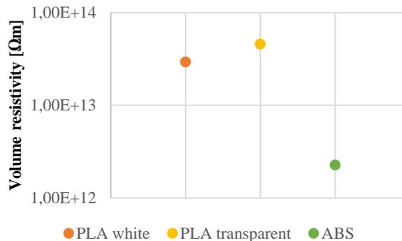
Figure 9. Volume resistivity of ABS and PLA
