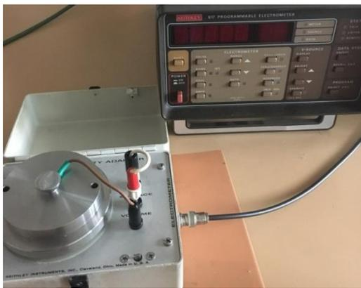
Figure 5. Volume resistivity measurement
