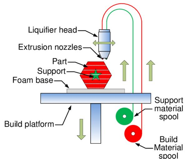
Figure 1. The principle of FDM printing proces [1]
