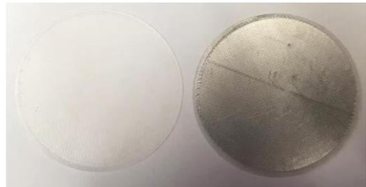
Figure 3. ABS samples: plain (left), with contact pads (right)
