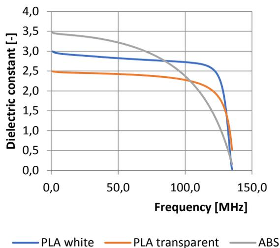
Figure 7. Frequency dependence of dielectric constant of ABS and PLA
