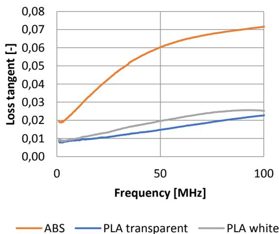
Figure 8. Frequency dependence of loss tangent of ABS and PLA
