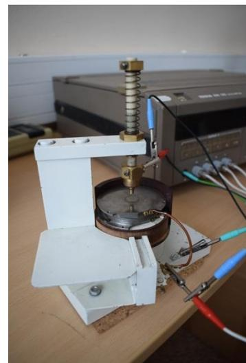
Figure 4. Dielectric constant measurement
