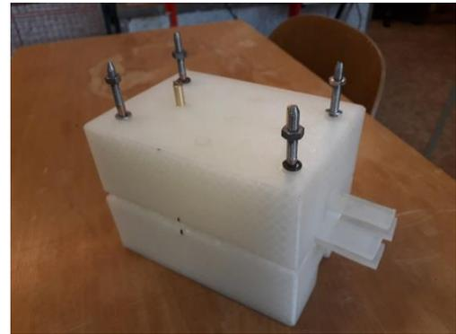
Figure 6. System for dielectric strength measurement
