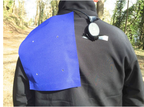
Fig. 9. Image of jacket, which comprises the textile antenna which is covered by the blue fabric and a GPS mouse.
