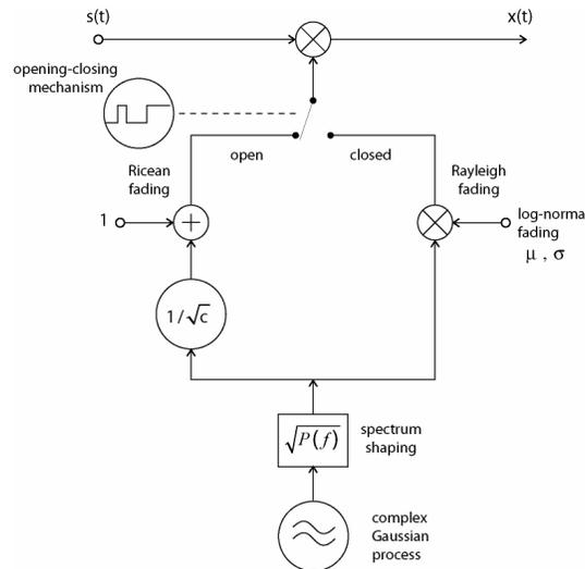
Fig. 3. Model of a frequency-flat fading satellite channel
