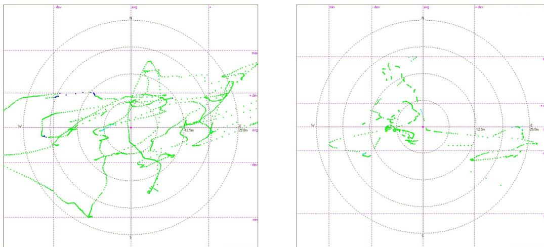
Fig. 9. Stationary GPS observations record and deviations for non-differential measurement (left) and with use of differential corrections from GOPE station distributed via Internet connection.
