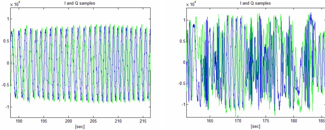
Fig. 1. Inphase (blue) and quadrature (green) output samples of GPS L1 correlator for measurement without user move (left) and measurement affected by user indoor movement (right).
